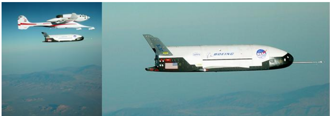
Figure 4. Two of three X-37ALTV flights used an air data boom; The third flight flew without an air data boom using CADS to support both primary and redundant air data requirements. (Photos courtesy of The Boeing Company)
