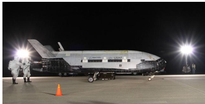
Figure 5. The X-37B demonstrated many technologies by successfully completing the first fully autonomous deorbit, re-entry, and runway landing at VAFB, December 3, 2010. (Photo courtesy of The Boeing Company)
