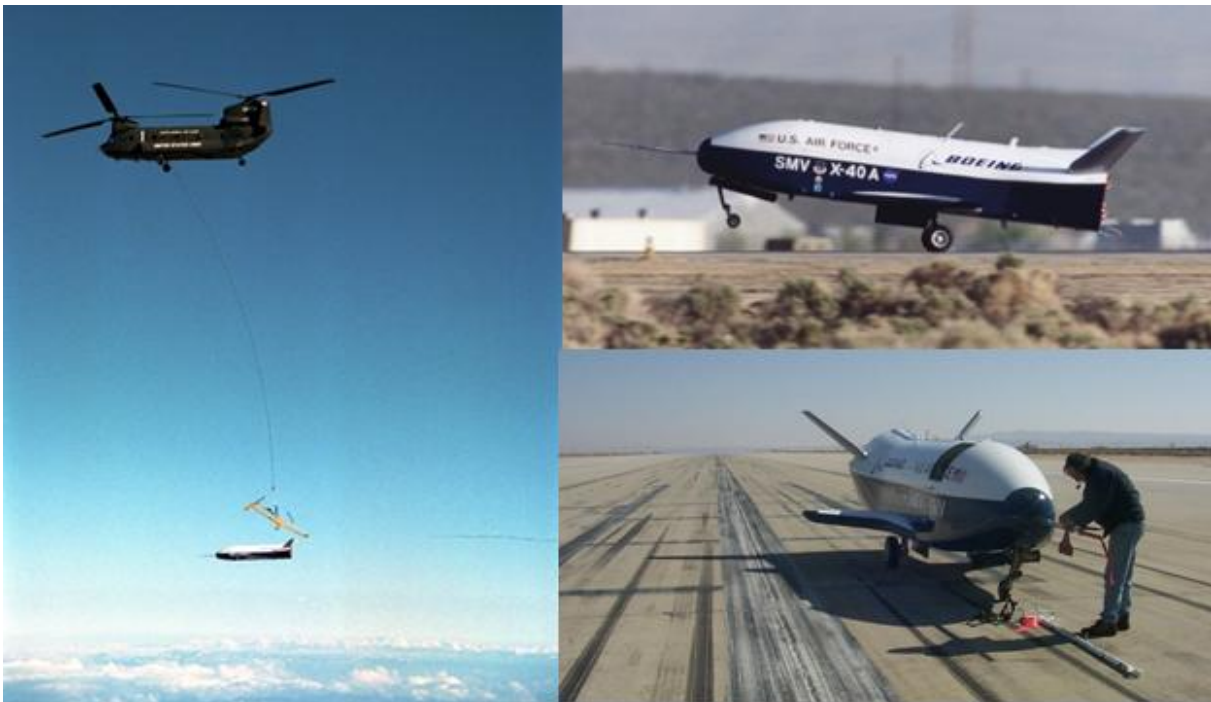
Figure 2. The X-40A Flight Program validated GNC algorithms, subsystem math models, and the methods for autonomous vehicle test and flight operations. (Photos courtesy of The Boeing Company)
