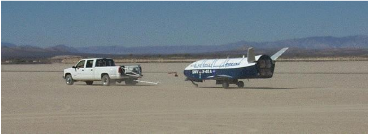
Figure 3. The concept of captive tow and free release was developed during the X-40A program since there wasn't a remote pilot capability with which to conduct dynamic taxi tests of the landing gear or GNC related subsystems. (Photo courtesy of The Boeing Company)
